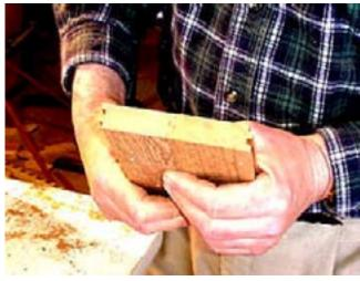
This time, it is right on. So remember, if the "B" side is low, raise the bit. If it is high, lower the bit. Literally, this setup should take no more than a minute or two and it will save you many minutes of planing uneven boards.
