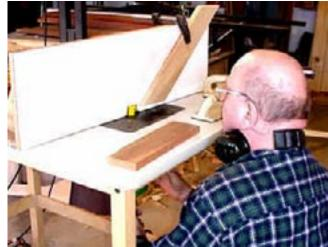
Now set the router height to the mid-point as marked on a scrap board. You don't have to be accurate. This is a starting point only.
