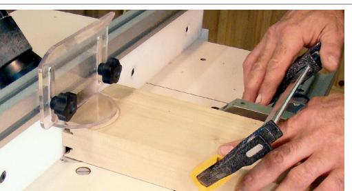
Make a test cut and check the set up. Machine a test piece.
